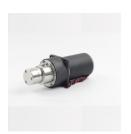
MG200XK / DC24 Magnetic drive gear pumps, the use of DC brush motor as the driving force, and the outer magnetic ring Motor shaft rare earth permanent connection, magnetic drive gear pump. Its advantages are simple structure, small size, large torque, by changing the voltage adjustment Motor Rev., to achieve flow regulation. MG200 full range of gear pumps are configurable brush motor.
